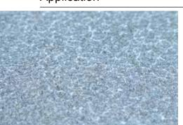
The surface must be dry, clean and firm, free of fats or oils. Shake the container well before using and applying Primacem GRIP to the surface with a brush or roller. Between 15 and 30 minutes, depending on the environmental conditions and the absorption of the support, it can be applied to the plaster, plastering.
